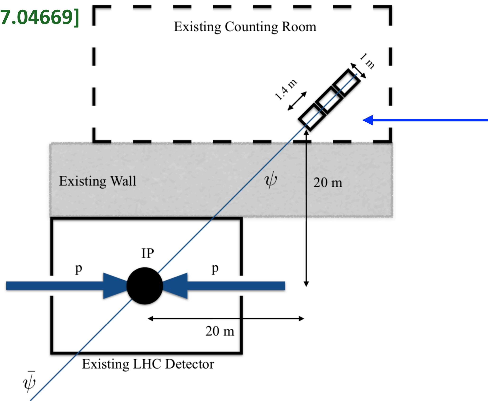
1 m × 1 m × 3 m plastic scintillators array with 3 sections (pointing to CMS IP), each containing 400 5 cm × 5 cm × 80 cm scintillator bars coupled to PMT. 33 m away from CMS IP.
